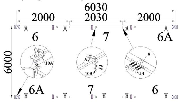
**Option B:** Welding angle seat to fix the square tube rails to the top of container.
