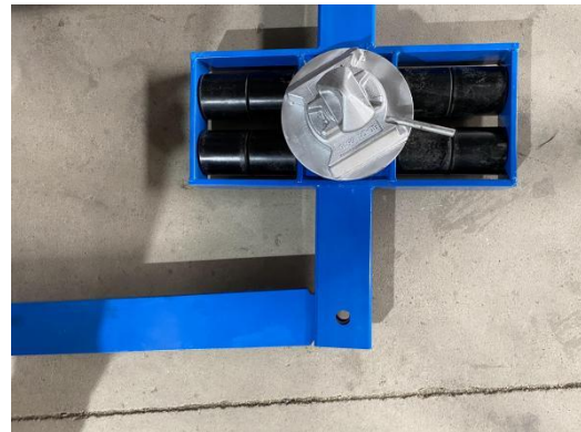
Align the CR-E16 body with the connecting arm holes
