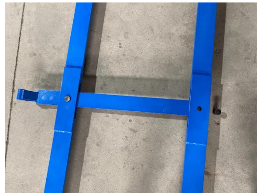
Install the CR-E16 handle connection arm and secure it with a pin
