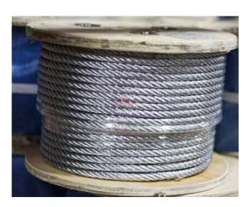
Store wire rope in a spool on a drum. Storing wire rope loose risks the rope getting tangled, birdnesting (or birdcaging), and developing kinks.
