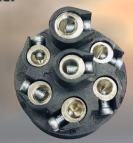
3. Tighten screws to keep wiring in place and reinstall housing. Your power cable should have 7 good connections now and be functional.
